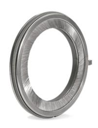
The Sentinel FBS is intended to be a drop-in replacement for a standard carbon ring seal. The brush serves as the primary shaft seal while a carbon element provides face sealing in the turbine's casing. Users have found that by utilizing the FBS, the interval between seal replacement increased more than 3x to an average 3 to 4 year life span.
